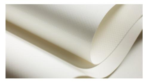
With its weight and tensile strength, Polyplan Hall PVDF is close to a Type I membrane, but optimized in its efficiency for industrial applications. PVDF is especially dirt repellent. Our PVdF lacquer can be normally welded with hot-air, hot-wedge or high-frequency machines. High-tenacity polyester base fabric in Type I weaving style with flame-retardant finish.
