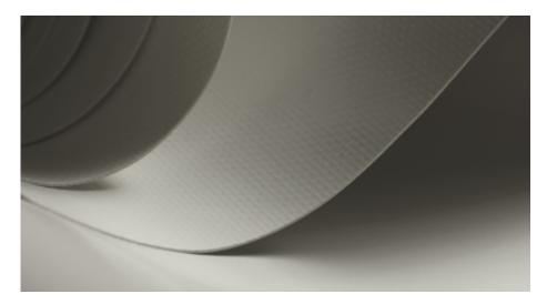
Type I membrane for the storage of biogas designed for applications with FR-requirements. Suitable as inner membrane for double membrane gas holders or as biogas bag mounted on a building for weather protection. Base fabric made of high-strength polyester yarns, coated on both sides with a specific PVC layer with biogas-resistant and flame-retardant formulation.
