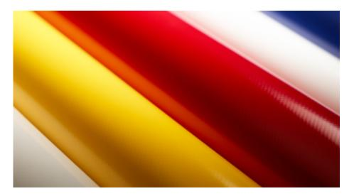
High-strength polyester fabric coated on both sides with a specific soft-PVC coating and UV-shield. Thanks to the special surface sealing, durability and best dirt-repellence are ensured. This tarpaulin meets the requirements for swap bodies as defined in DIN EN 12 641-1.
