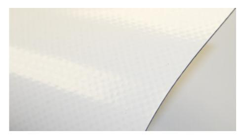
High-strength polyester fabric, blockout on both sides, coated with soft-PVC. The membrane has a fungicide finish, is lacquered on both sides and flame retard according to EN 13501-1. High-gloss surface.
